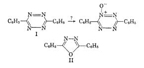
The starting material I, prepared by an improved method,<sup>3</sup> was allowed to react with an excess of peracetic acid at  $50-60^{\circ}$ : the initial redpurple color of I disappeared giving a colorless solution, from which 2,5-diphenyl-1,3,4-oxadiazole<sup>4</sup> (II) was isolated in good yield.
